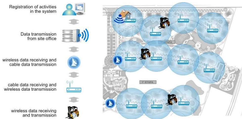
Figure 4: Step by step of transmitting information and coverage area of the wireless network in the construction site
